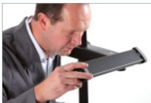
The wide-band visor with integrated reticule can be adapted to different heights thanks to horizontal adjustment.
