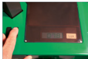
The digital luxmeter is used to determine the glare value of the low beam and the illumination strength of the high beam quickly and easily.
